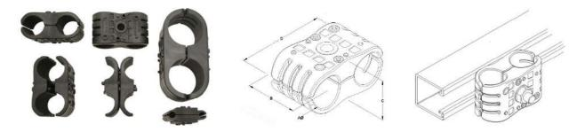
All two piece double clamps are designed to precisely fit the cable diameter. These GCA Ltd double clamps are manufactured in high grade polypropylene and UV stabilised to prevent degradation or breaking. For 'flame retardant' clamps to UL94V-0 (0.8mm) LSF Halogen and Phosperous free material state '2P-DW007.5mm - FR'
